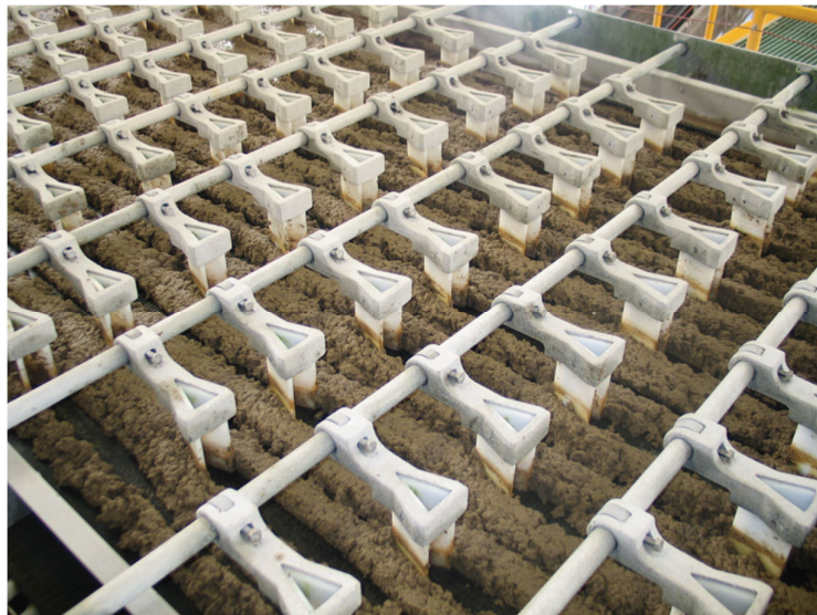
Belt press operations with Zetag 7583 flocculant bead
